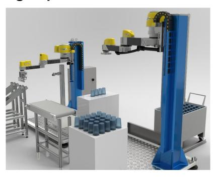
As an example of automated boxing, a constructing with two SCARA SPIN robots from Campetella with low space and cycle time requirements shows the automated taking out, stacking and boxing of cups with different labels.
